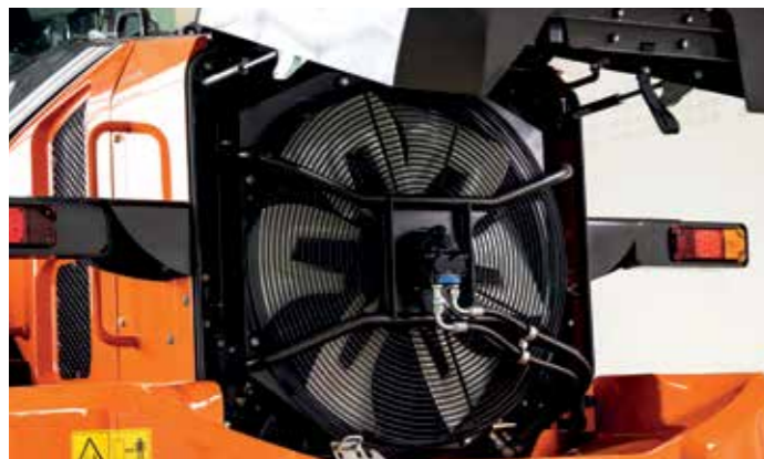
Intelligent fan operation system prevents radiators clogging.
