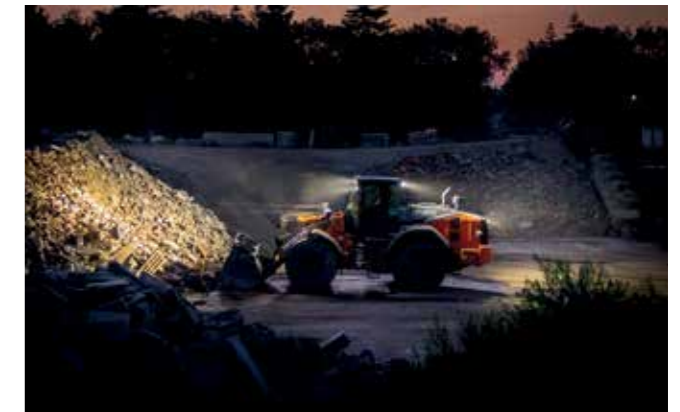
LED work lights improve visibility in challenging conditions.
