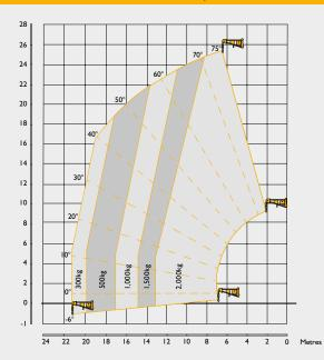
555-260R LIFT PERFORMANCE - 1000KG SLEWING MAN PLATFORM WITH OUTRIGGERS DEPLOYED
